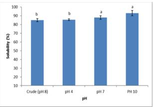
Figure 2. Solubility of shortfin scad waste hydrolysate (SWH) at different pH level (pH 4, pH 7, and pH 10) as compared to crude (pH 8.0). Different letter (<sup>a-b</sup>) means significantly different (p< 0.05) in the mean of sample. Data reported are means values  $\pm$  standard deviations.
